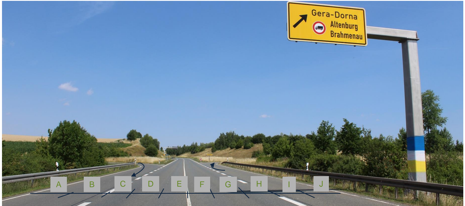
Fig. 8: Sampling positions (S3) on a road (A-J), points A and B in the acceleration track and I and J in the deceleration track (B2 near Gera-Dorna).
