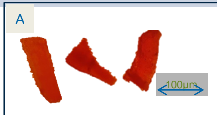
Fig. 12: Light microscope image of PVC particles (A), scanning electron microscope image of TRWP (B), and incrustations magnified (C) (Kreider, et al. 2021).
